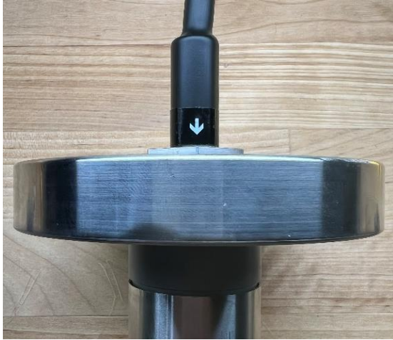
Figure 7. The outlet port aligns with the sticker shown.
